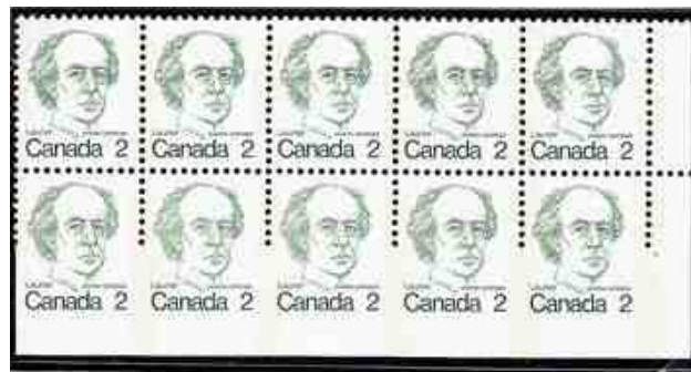
Lower right corner block of 10 2¢ stamps, part imperforate, caused by the one-line H-comb perforator missing the last strike
